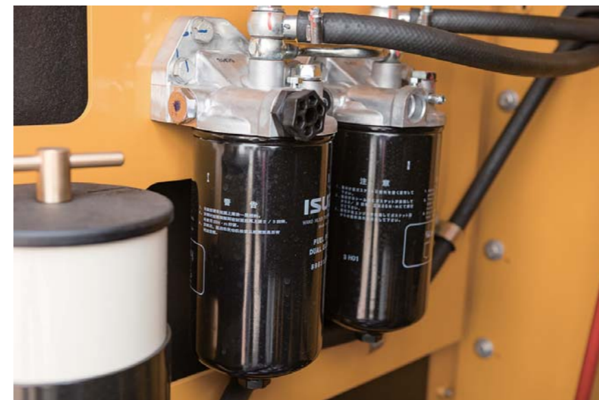
High-capacity multi-stage filter system
