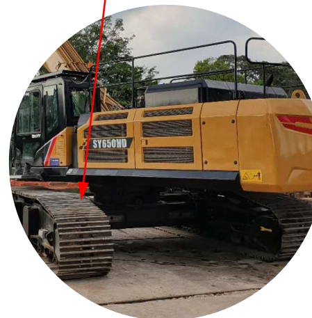
4. Design with hydraulic extension track gauge and lower chassis GC, much more compact for transport and with super stability and higher safety for operate.
